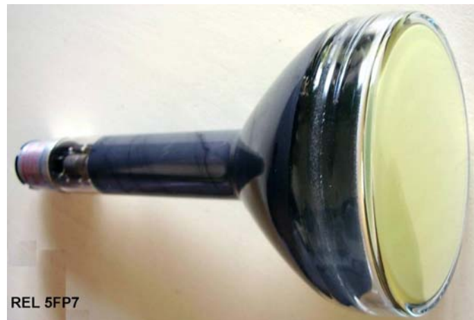
Fig. 18 - Typical radar CRT displays used P7 phosphor type, characterized by blue trace followed by yellow persistence. Probably 5FP7 was the most diffused 5-inch CRT through the war. This sample was built by Canadian REL. Click to enlarge.
