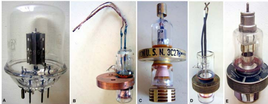
Fig. 17 - High-frequency transmitting tubes designed during WWII for pulsed operation in IFF or in navigation equipment. A) 826 was used in the IFF interrogator of SCR-268 radar. B) British CV155 ‘milli-micropup’ could generate 40 kW pulses at 1200 MHz. C) National Union 3C27B was an American derivative of CV155, rated for 10 kW pulse power. D) RCA 4C28 was designed for the pulse transmitter sections of the SHORAN navigation system. E) 4C29 was registered to Canadian REL and used by Canadian Air Force. Click to enlarge.
