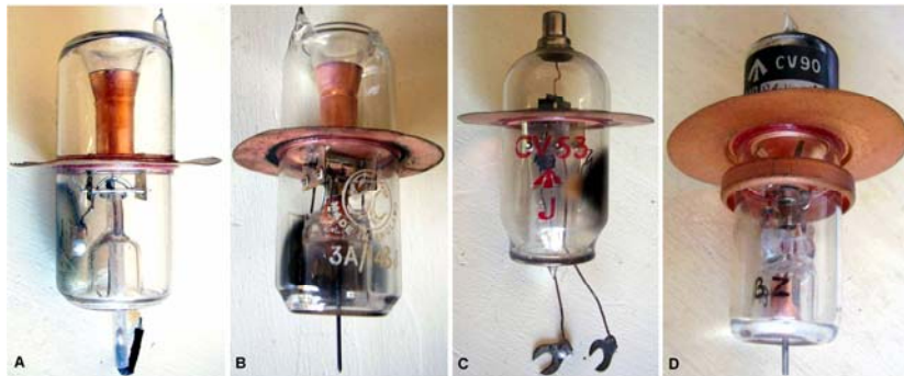
Fig. 2 - Samples of British planar receiving tubes. A) CV16 early planar triode. B) CV88 was designed to operate up to 600 MHz. C) CV53 was a simplified variant usable up to 400 MHz. D) CV90 was capable of operation up to 3 GHz. It was the forerunner of 'rocket' tubes, so called for their shapes. Click to enlarge .
