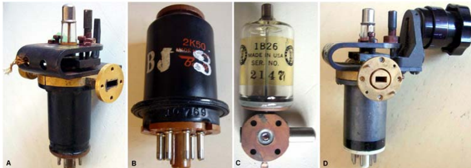
Fig. 16 - Tubes developed for the K-band. A) 2K33 was manufactured by Raytheon, starting from a design developed at Clarendon University. B) 2K50 was a fine WE design using electronic tuning. C) 1B26 TR switch was a scaled down 1B24 . D) This OK291 was one of the many frequency variants of 2K33. Click to enlarge .
