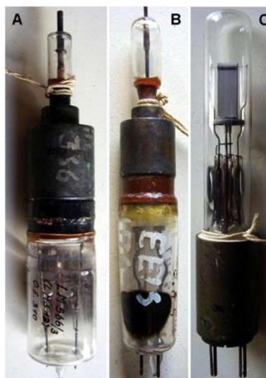
Fig. 16b - Rarest WWII German magnetrons. A) LMS 12 magnetron was used in the few units of Berlin-D, 3 cm set, made before the end of the war. B) The 1.65 cm LMS 13 was just in the evaluation phase, as the RM4025 in C. For more information refer to the article on German WWII magnetrons . Click to enlarge .
