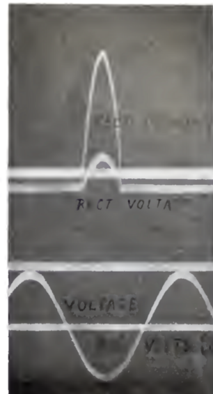
Fig. 11. Rectifier Charging Ignition Cells at 6.2 Amperes Direct-Current Voltage Across Battery and Regulating Resistance
